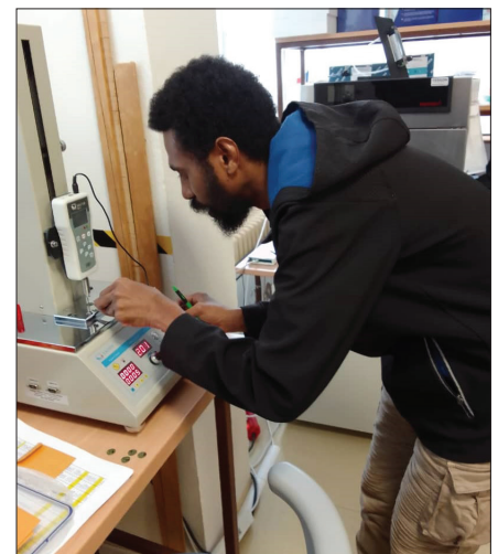
▲ Dr Maraia measuring leaf toughness in the molecular laboratory using an electronic penetrometer.
